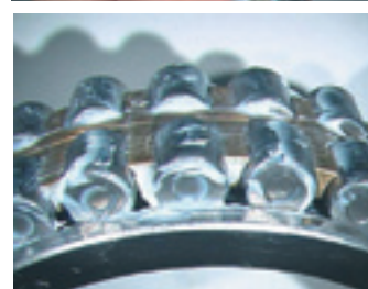
Photo. 6.2 Filling grease into cylindrical roller bearing
